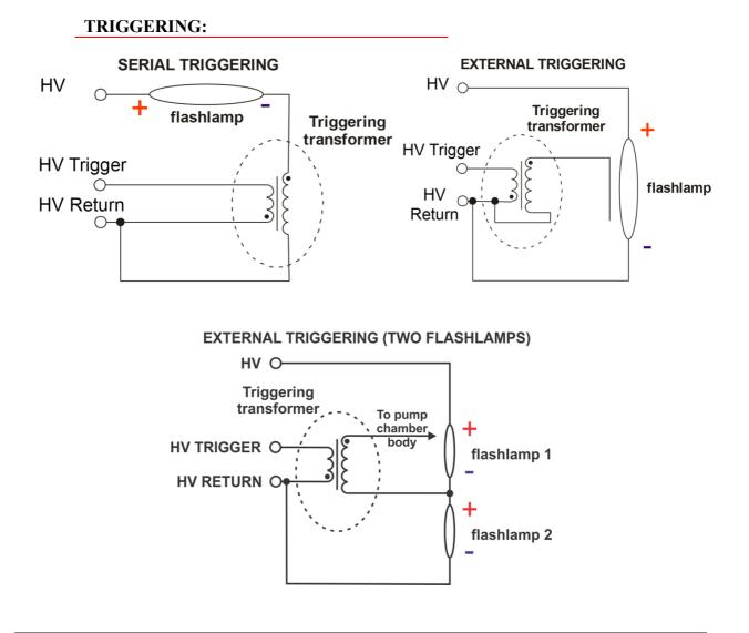
**Grounding policy** HV Return is not connected to the Case ground. In the case of need the customer can interconnect them by himself. Other grounding policies are available on request **Warning!** This equipment produces high voltages that can be dangerous. Don't be careless around this equipment.
