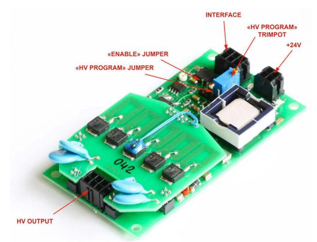
There are three Molex microfit connectors, two jumpers and one trimmer potentiometor on Pockels cell driver board. The description is below.
