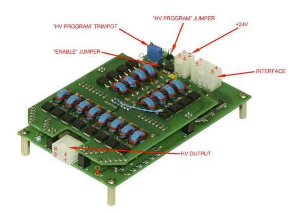
There are three connectors at Pockels cell "driver" board. Hereafter is description of corresponded female connectors (supplied with the board)
