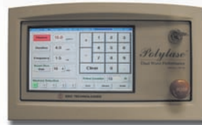
LASER CONTROL PANEL
