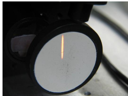
Image of 1W/1470 nm laser diode beam transmitted through cylindrical lens.
