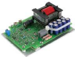
CAPACITOR CHARGER BOARD - PBZ-0204
